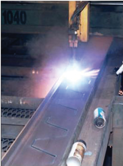
Fig. 1-2. Cutting of a castellated pattern.
